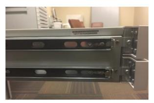
3.9.7. While pulling on the front releases, pull the drawer out to the second stop. This exposes the cable arm cover. This requires a little force, ensure you do not use extreme force. If the cable arm cover fails to be fully exposed, check the rails are retracted fully.
