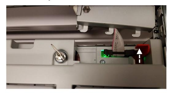
3.9.10. Locate the release mechanism under the drawer. Pull and hold the release mechanism out towards the side of the drawer.
