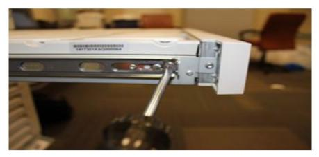
3.9.6. To remove a double-deep drawer you must loosen the slotted screw on the bottom rail. Then pull all four of the front releases at the same time
