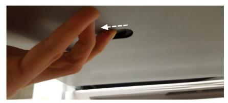
3.9.11. While pulling the release mechanism, all the bins can now be opened.
