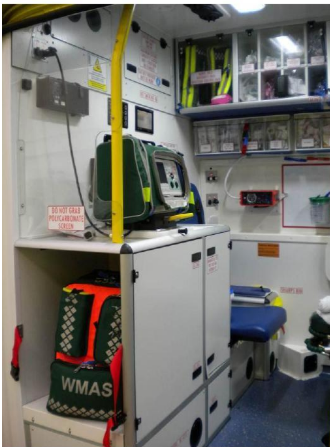
o/s bulkhead cupboard with defib bracket
